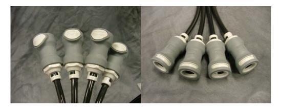
To connect ink tubes first separate them from each other at the ends. Initially you should separate about 4" (10cm) to allow for connection to fittings. Push tubes firmly but carefully over ink ports on the reservoir using caution not to break fittings. Next, install the quick connects to the other end of the tubing using the same method. Emery cloth can be used to grip the tubing better.
