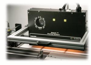
The Speed-Dri Model 5061 provides instantaneous infrared and convection technologies to dry ink printed on target areas up to 4" (102 mm) wide. Depending on the application, web speeds of up to 500 feet/min. can be achieved.
