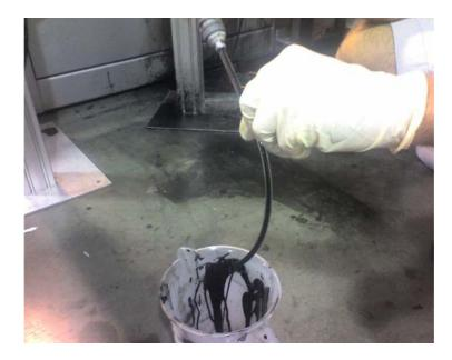
Disconnect the priming piece and that specific out-port line has been primed. Repeat this process until each of the out-port lines on the Bulk Supply Station have been primed. You are then ready to attach the lines to the IM1 cartridges (while the cartridges are in their specific print stall), as pictured below.
