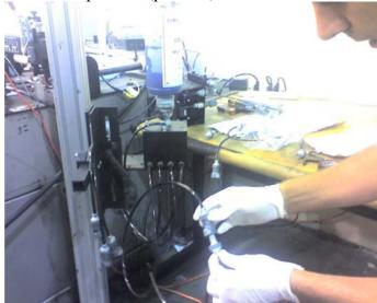
Then allow at least 5 mL of ink to run through the priming piece into a waste container.
